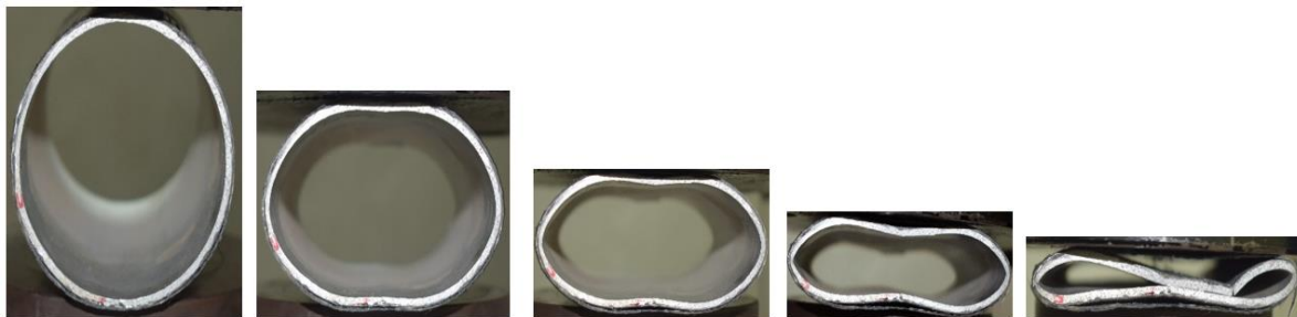
Figure 1: Progressive deformation of aluminium-glass fabric reinforced composite hybrid tube
