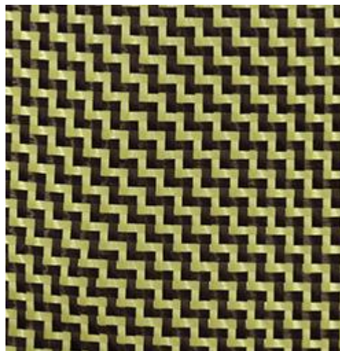
Figure 1: Carbon kevlar twill woven fabric
