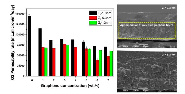
Figure 1:  $O_2$  Gas barrier properties of the TPU/graphene composites loaded with graphene of different thickness or number of layers and their corresponding cross-sectional SEM images. (G<sub>t</sub> indicate graphene thickness in nm).
