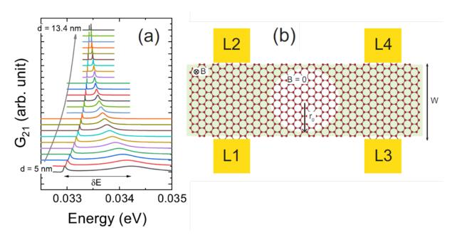
**Figure 1:** (a) Conductance spectra through the MQD for various MQD-edge distances. Each curves are calculated from the S-matrix approach between L1 and L2 leads. (b) Schematic model of the system. Uniform magnetic fields are applied to the graphene Hall bar with four leads, and screened out in the circular region, resulting in the MQD.
