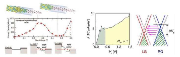
Figure 1: Quantum-hybridization NDR from 1D halide perovskite nanowires [1] (left) and graphene electrode-based 2D vertical tunneling transistors [2] (right).
