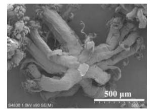
Figure 1: SEM image of CNTs on the beads.
