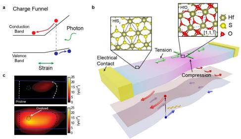
Fgure 1: a) Charge-funnel Selective concept. b) oxidation lead to lattice mismatch at the interface between HfS2 and HfOx creating a strain gradient which modulates the bandgap. C) Enhanced photoresponse is observed in proximity of the oxidised area as a result of chargefunnelling.
