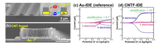
**Figure 1:** (a, b) Side-view SEM images of the CNT forests on Au electrodes. CV results of (c) Au-IDE (reference) and (d) CNTF-IDE with the K<sub>4</sub>[Fe(CN)<sub>6</sub>] (100 µM) in KCI (100 mM) at the scan rate of 10 mV s<sup>-1</sup>.
