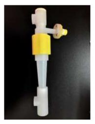
Figure 1: Hydrocyclone used as a classifier to separate graphite and graphene.
