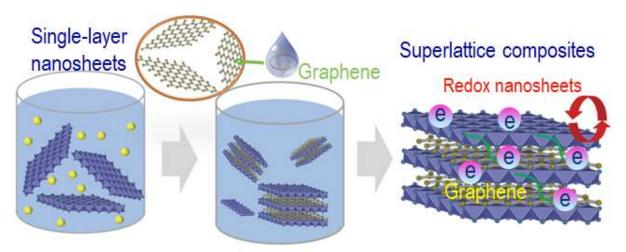
Figure 1: Molecular-scale hetero-assembly of single-layer nanosheets and graphene for superlattice-like composites.
