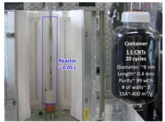
**Figure 1:** Semi-continuous, high-yield production of 500 µm-long, 99 wt%-pure few-wall CNTs by FBCVD [4].
