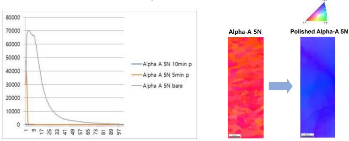
Figure 2: (a) Oxygen content in polished Cu foil (TOF-SIMS) (b) phase orientation of annealing Cu foils (EBSD)
