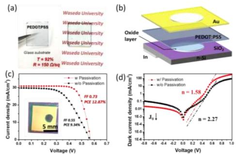
Figure 1: Solution-based PEDOT: PSS-/n-Si heterojunction solar cell with 1-min surface passivation.
