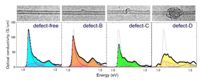
**Figure 1:** Absolute optical conductivity of a semiconducting (9,2) at three different defects as well as a defect-free region. This shows how the gap transition and exciton lifetime depend on the type of local defect [2].
