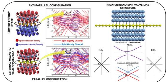
**Figure 1:** Spin-dependent charge density mapping (left) and bandstructure of Ni/Graphene/Ni nanostructure (middle). When the magnetic moment between upper and lower nickel slabs is antiparallel (parallel), the Dirac cone of graphene is open (close). The Klein paradox on graphene need to be reconsidered by proposed partially sandwiched structure of graphene nano-ribbon with nickel layers from upper and lower side (right).
