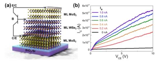
Figure 1: (a) schematic of an npn double HBT (b) output characteristics of a fabricated npn double HBT
