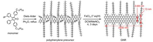
Figure 1: An example for bottom-up solution synthesis of graphene nanoribbons.[3]
