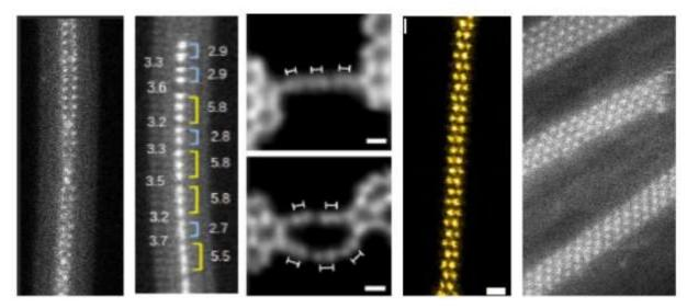
**Figure 1:** Examples for one-dimensional structures: (Left to right) Eu double atomic chains, iodine mono-atomic chains, carbon chains, MoSe nanowire, WS<sub>2</sub> nanoribbons.
