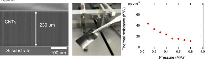
Figure 1(a): SEM image of CNT sheets after annealing at 2400 °C. (b): Photo image of CNT sheets. (c): Thermal conductivity of CNT sheets dependent on pressure.
