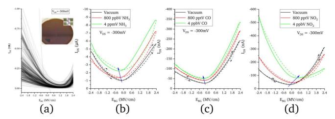
Figure 1: (a) Input characteristics of 524 ncGFETs measured in ambient air, inset shows 2" wafer with the respective devices. Input characteristics of different devices under influence of (b) NH<sub>3</sub> (5.0), (c) 1,000 ppm CO in dry technical air, (d) 1,000 ppm NO<sub>2</sub> in dry technical air. Concentrations have been calculated from the vacuum pressure in the chamber
