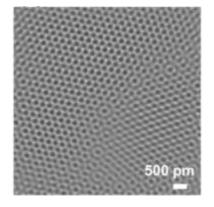
**Figure 2:** Grain boundary of graphene synthesized by high-throughput plasma CVD
