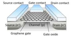
**Figure 2:** Schematic illustration of a graphene-gate transistor (sensor)
