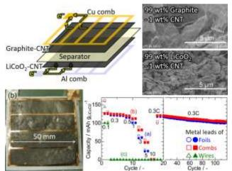
**Figure 2:** Lithium ion full cell with LiCoO<sub>2</sub> cathode and graphite anode based on CNT 3D current collectors [6].
