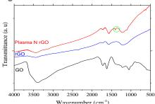
**Figure 1:** FTIR spectra of GO, rGO and plasma NrGO.
