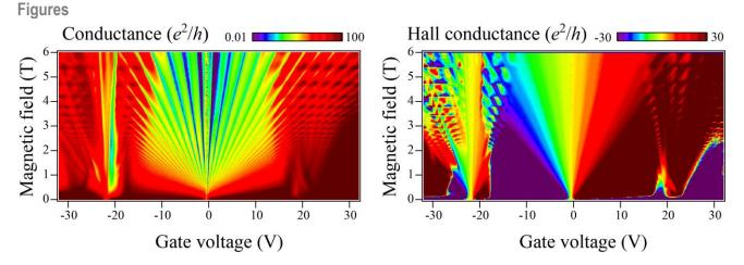
**Figure 1:** Longitudinal conductance and Hall conductance as a function of a gate voltage and a magnetic field applied perpendicular to the substrate at 6 K in single-layer graphene/hBN superlattice devices.
