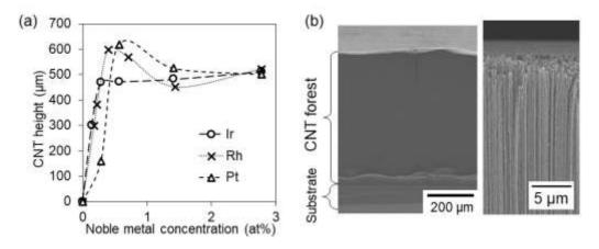
**Figure 1:** (a) Height of CNT forest (Grown within 10 minutes) vs Atomic concentrations of noble metal (Circle: Iridium, Cross: Rhodium, Triangle: Platinum) added into iron catalyst. (b) SEM images of CNT forest from Rh 0.4 at% catalyst (inset: Photograph from top of the forest).
