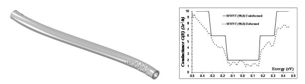
Figure 2: Simulations of a MWCNT where the two ends of the tube have been misaligned by 30 nm.
