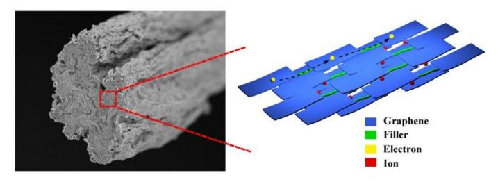
Figure 1: SEM image and scheme of graphene composite fiber.
