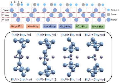
**Figure 1:** Various stacking arrangement on Ni/hBN interface (upper). Some representative figures as the results from thirtysix configurations. From left to right, the total energy increasing from the most stable to the unstable structure (lower). The combination of top-fcc on the top side and top-hcp on the bottom side are the most stable structure.
