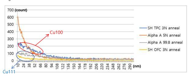
Figure 1: Oxygen content in annealing Cu foil (TOF-SIMS)
