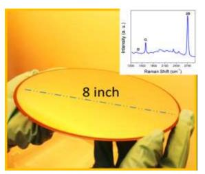
**Figure 1:** Graphene, grown on 200 mm Ge(100)/Si(100) wafer. A typical Raman spectrum of the Graphene is presented in the inset of Fig.1
