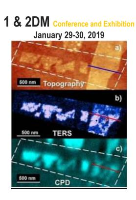
Figure: AFM topographic, TERS and surface potential images of WSe2 flakes
