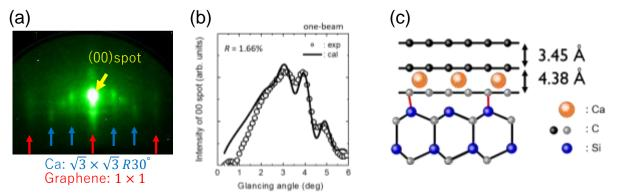
**Figure 1:** Structure analysis of Ca-intercalated bilayer graphene on SiC(0001). (a) TRHEPD pattern, (b) experimental rocking curve (circles) and theoretical curve (line), (c) structural model determined by TRHEPD.
