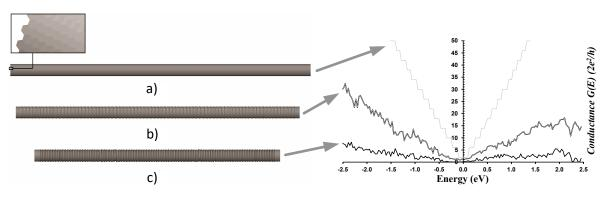
**Figure 1:** Model reproducing a MWCNT: a) in the undeformed configuration, b) compressed axially by 20 nm, c) compressed axially by 50 nm. The inset shows a magnification of the outermost wall revealing the hexagonal cells.
