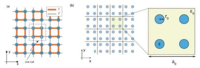
**Figure 1:** (a) Schematic lattice structure of the 2D SSH model. The model is specified by the intracellular hopping  $\gamma$  and the intercellular hopping  $\gamma'$ . (b) Schematic of the dielectric crystal mimicking the 2D SSH model. The unit cell consists of four identical dielectric cylinders of radius  $r_0$  placed at (±0.25, ± 0.25) $r_0$ . The lattice constant is  $a_0$ .
