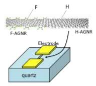
**Figure 1:** Illustration of a diode using a heterojunction of F-AGNR and H-AGNR.
