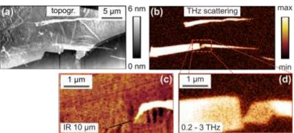
Figure 1: The conductivity of single layer graphene can be visualized through the s-SNOM contrast in the IR and THz spectral range. High reflectivity in the IR shows highly conductive areas, while those areas that are reflective in the THz spectral range are expected to have higher conductivity than the non-reflecting surroundings but lower conductivity than the areas that reflect IR light.
